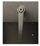
Rotate handle clockwise to return the balls to the blower chamber. Rotate handle counter clockwise to return the tray to the gaming position.
